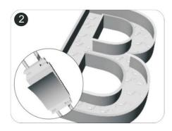
To Peer off the adhesive tape on the back of the module, and lightly stick to installation slot for initial positioning.
