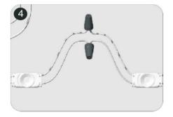
When the modules are connected in series, the positive and negative wires of the modules are pe eled separately for 10mm and then connected with terminal, and do waterproof, insulation, anti - short circuit and anti - corrosion treatment
