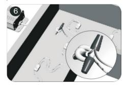
The positive and negative wire need to be correctly connected to the positive and negative terminals of the power supply output.
